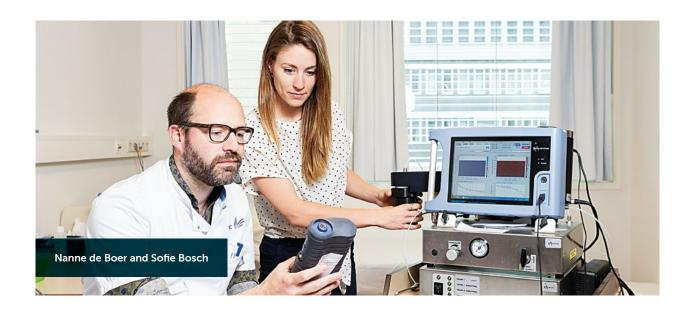
Faecal samples were measured using an advanced eNose apparatus, the G.A.S. Flavourspec, which is based on gas chromatography-ion mobility spectrometry (GC-IMS). The data were split into three sets, 70% for training and validation and 30% as test set. Supervised machine learning classifiers were used to provide statistical results.
