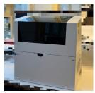
The advantage of the 4200 TapeStation System compared to the 2200 TapeStation System is that there is less loss of tape lanes and that more samples can be measured in a run . The 4200 TapeStation System makes it possible to quickly determine the QC of the DNA/RNA from 1-96 samples with wide range of ScreenTape applications, including assays for genomic and cell-free DNA.
